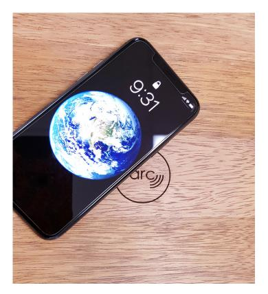
The ARC-H through surface wireless charger offers the ultimate in charging convenience. With a charging range of 15-30mm, ARC-H can be installed without the need to rout into the underside of the surface for surface thicknesses up to 25mm. Once installed ARC-H is completely hidden requiring a simple decal to guide placement of mobiles on the surface.
