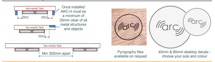
**INSTALLATION:** ARC-H has a wireless range 15-30mm, no routing is required for thicknesses up to 25mm.
