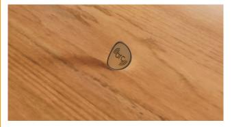
Position your wireless charging marker decal on the desk where you would charge your phone. Under desk / surface must be clear of framing, metal objects and metal structures.
